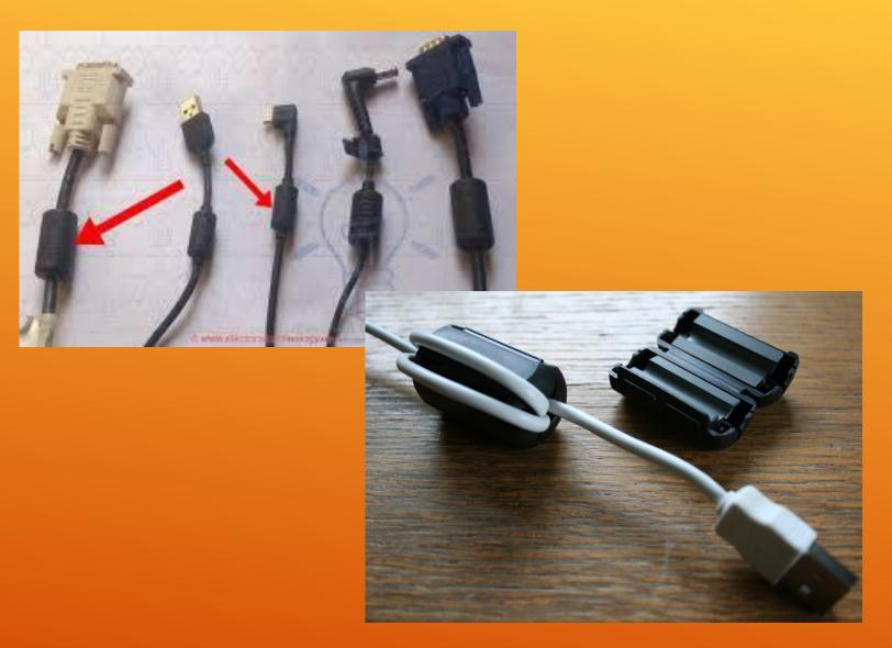
The most efficient and affordable solution to this issue is utilizing Ferrite
