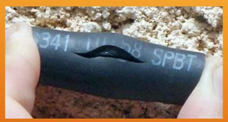
If the cable jacket becomes brittle and cracked, water could enter the cable, causing it to fail. You can also use electrical conduit to protect the cable from damage.
